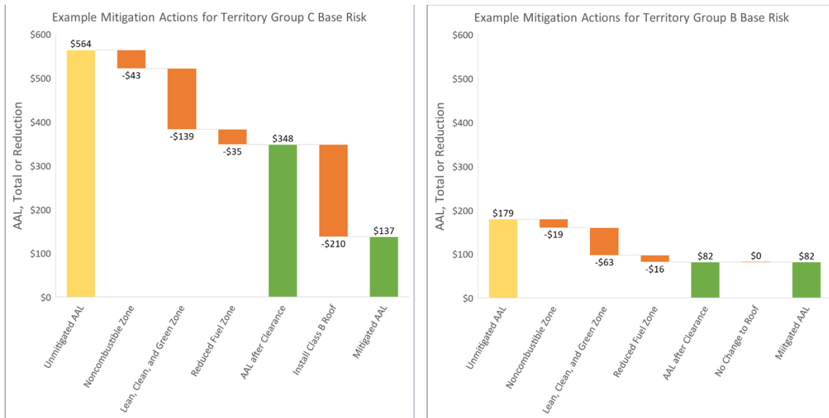
Figure 4.7. Sequential AAL and reduction for performing clearance, then upgrading roof if required
